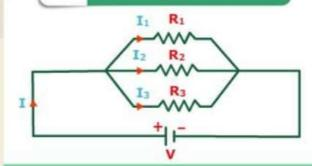
The sum of current passing through each resistance is equal to the total current coming from the battery.
